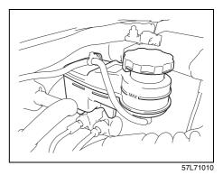
Check the clutch pedal for smooth operation and clutch fluid level from time to time. If clutch dragging is felt with the pedal fully depressed, have the clutch inspected by your SUZUKI dealer. If the clutch fluid level is near the "MIN" line, fill it up to the "MAX" line with SAE J1703 or DOT3 brake fluid.
